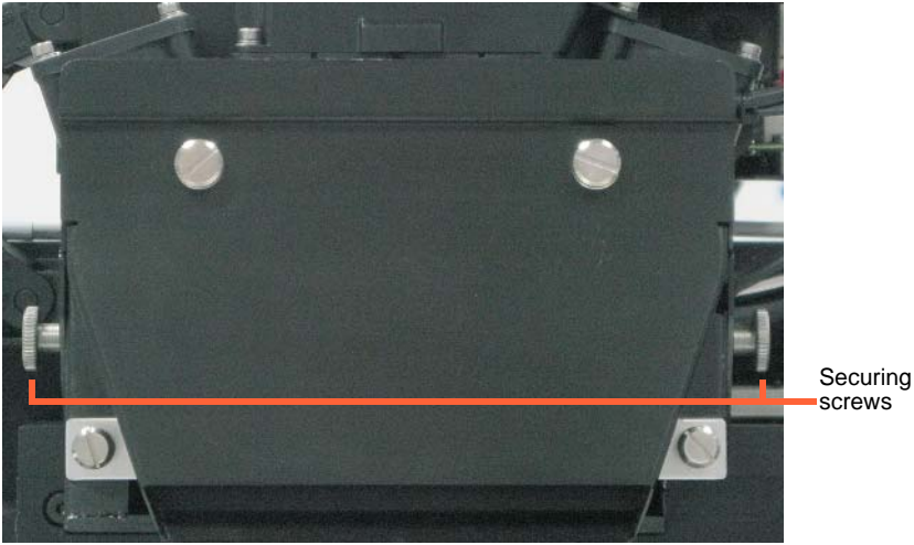
Figure 6-41: UV-lamp-assembly securing screws
