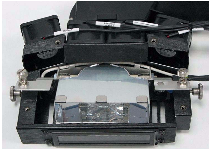
Figure 6-64: Removing the UV reflector from the UV assembly
