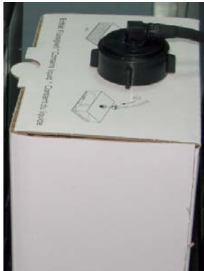
Figure 6-71: Waste container with drain tube attached
