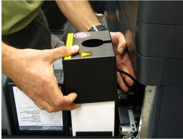
Figure 6-70: Removing the waste-container cover
