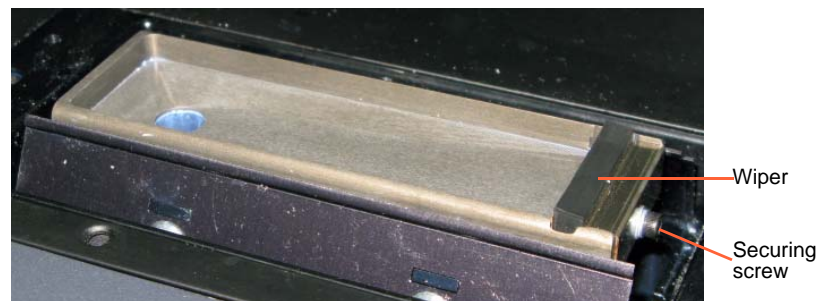
Figure 6-37: Wiper and excess-material drain
