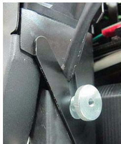
Figure 6-66: UV-lamp cable after replacing the assembly
