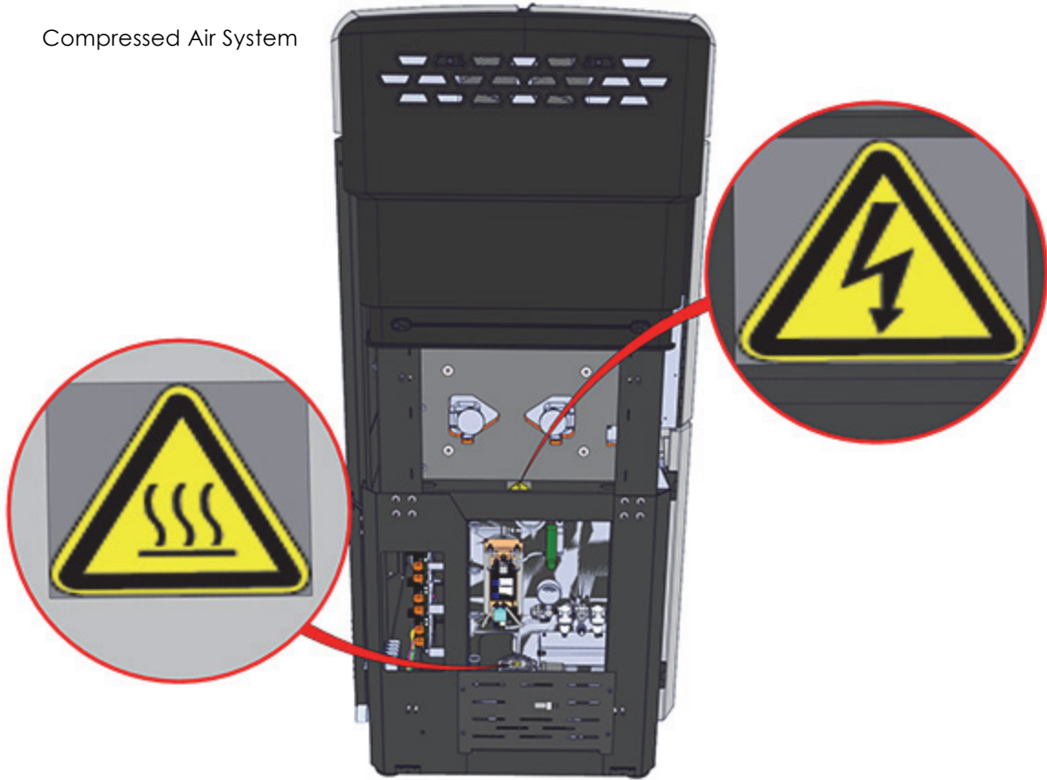
Figure 1-4: Air system safety label locations
