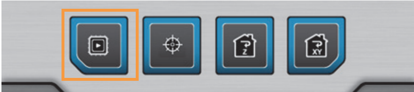
Figure 6-2: XYZ Tip Offset Calibration Button Location
